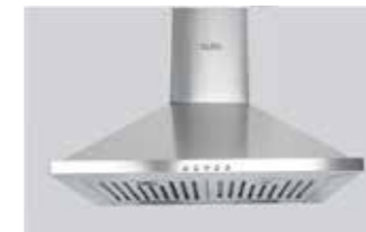
CH 6075 SS (60)* • Airflow 750/1000 m 3 /h • FRP housing • 2x40 W lights (750 m 3 /h) • 2x3 W LED candle bulbs (1000 m 3 /h)
