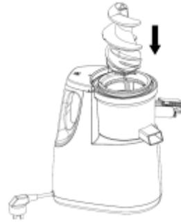
Align the triangle on the feeding tube with the unlock mark on the juicer bowl, then rotate clockwise, align the triangle with the lock mark so it is completely locked. Otherwise it will not start.
